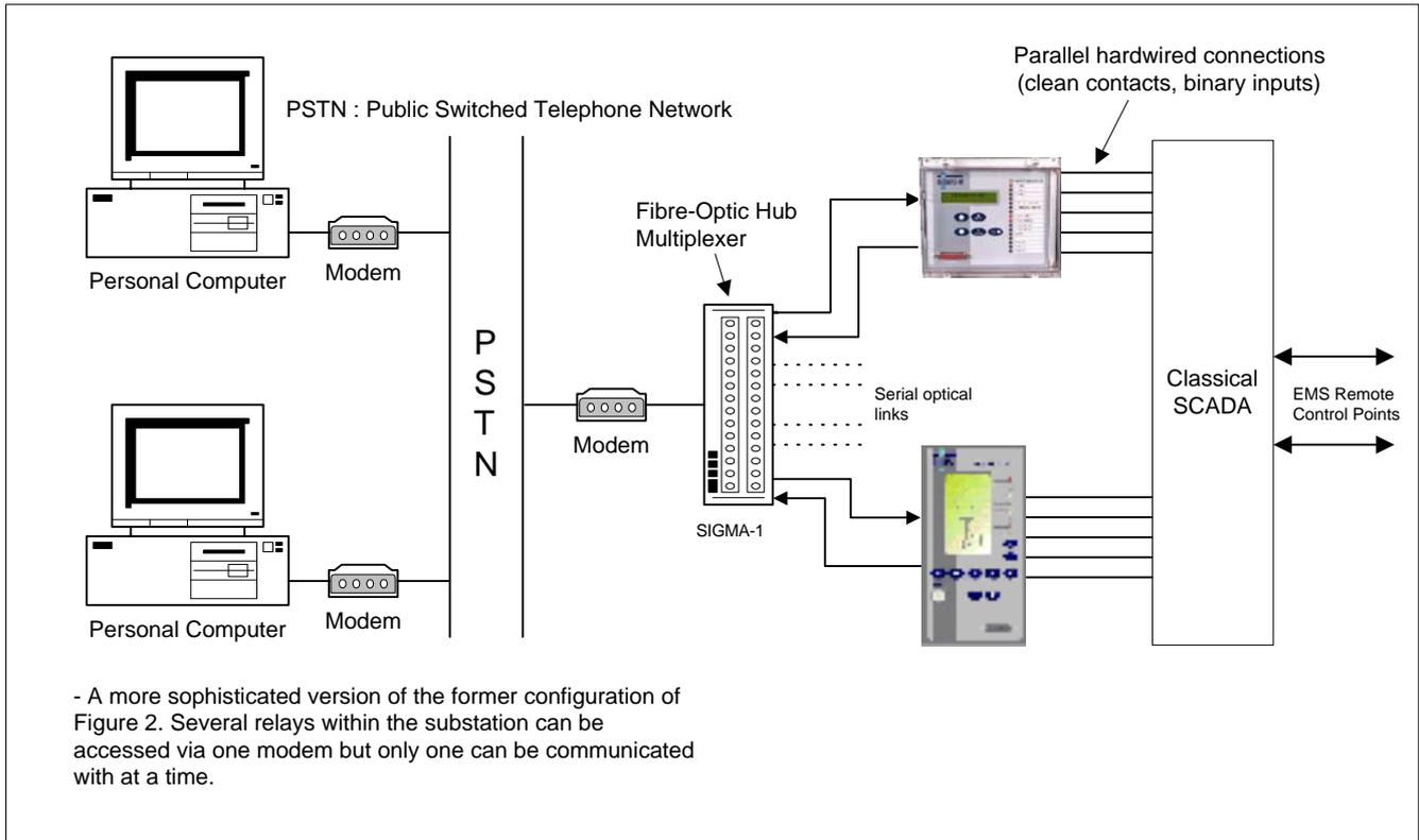
Figure 3 - Star Type Configuration (Using SIGMA-1 Multiplexer)
