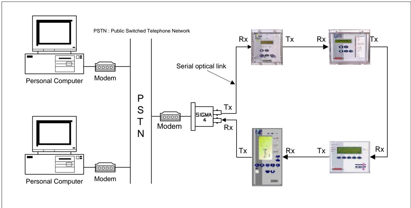
Figure 4 - Optical Ring Configuration (Using SIGMA-4 Fibre/RS232 Converter)
