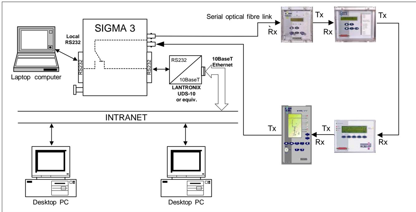
**Figure 7 – LAN Network connectivity using a SIGMA-3 + Lantronix UDS-10 or equivalent**
